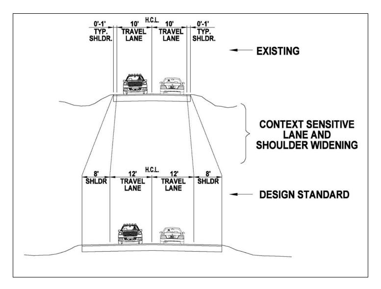
Comparison of existing typical section vs. design standard for Malden Turnpike, and recommended context sensitive widening in between.
